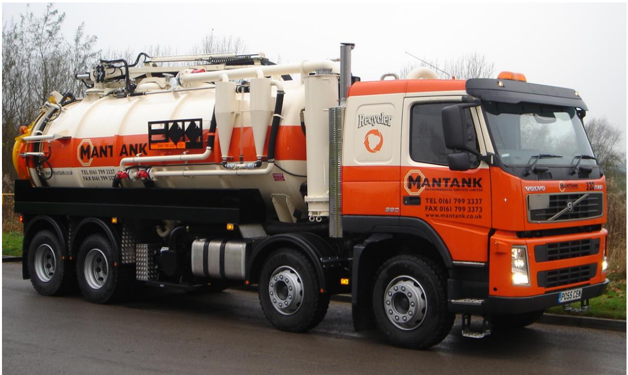
Dyna Combi System Power Pack, Water Recycling, Schlauchhaspel, Kassettenschlauch
